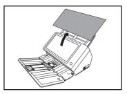
4. Pull the lock lever toward you and then fully open the panel unit.
