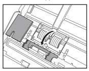
7. Gently close the panel unit. Press on both sides of the unit until you hear a click, which indicates the unit is locked.
