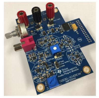
Figure 1. Analog Crossover Audio Plug-In Module
