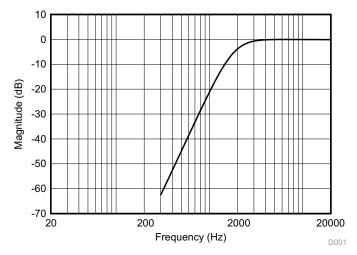
Figure 13. High-Pass Filter Frequency Response
