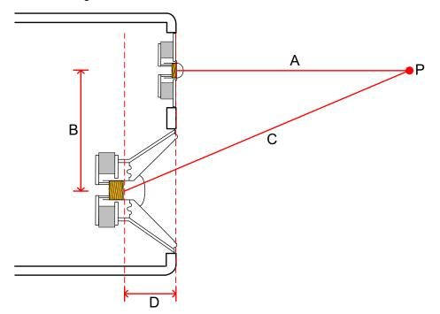
Figure 14. Cross Section of Two-Way Loudspeaker Requiring Delay Compensation
