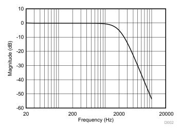
Figure 8. Low-Pass Filter Frequency Response
