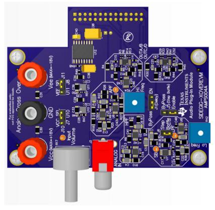
Figure 6. Analog Crossover Plug-in Module Controls
