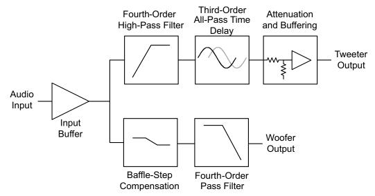
Figure 2. Analog Crossover Module Block Diagram
