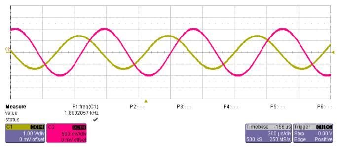
Figure 16. Example of All-Pass Filter Delay
