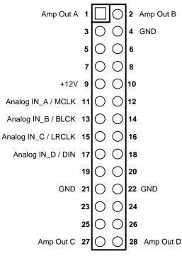
Figure 4. AIB Connector Pinout
