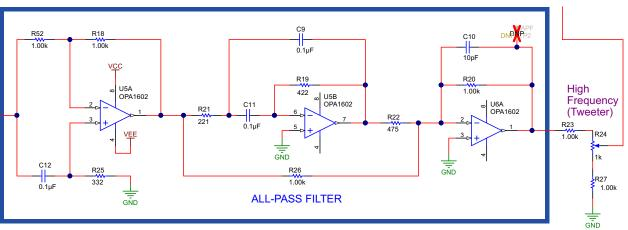
Figure 15 shows the schematic of the all-pass filter.
