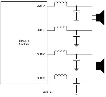
Figure 3. Class-D Output Drawings
