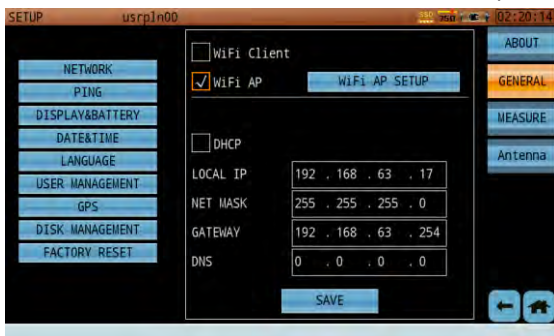
Figure 14-9 Setup S7200 as a WiFi hotspot
