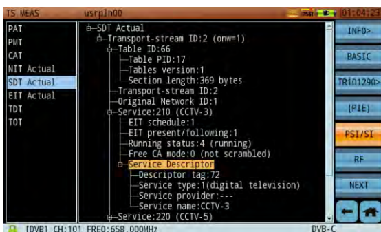
Figure 12-88 PSI/SI Analysis-SDT Table
