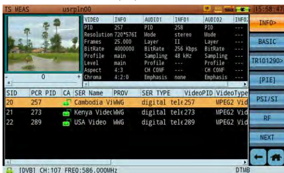
Figure 12-44 View image of DTMB signal
