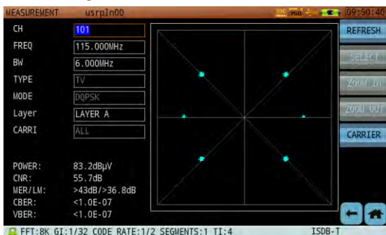
Figure 12-41 ISDB-T B Constellation
