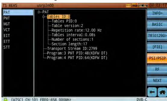
Figure 12-95 PSI/PSIP Analysis-PAT Table
