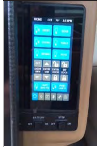
Figure 11-8: Bus step switch
