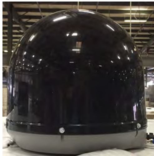
Figure 6-2: The dome satellite on top of the motorhome can be raised, allowing easy access to change dip switches to a new satellite provider.
