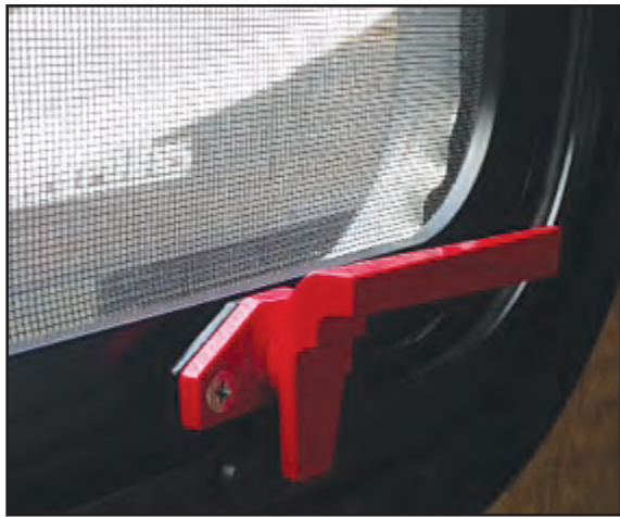
Figure 2-7: Emergency exit latch
