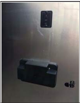
Figure 11-4: Electric Slide Tray Switch on cargo door
