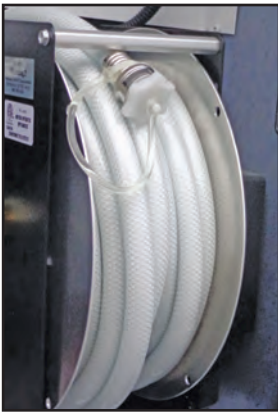
Figure 13-6: City water supply connection
