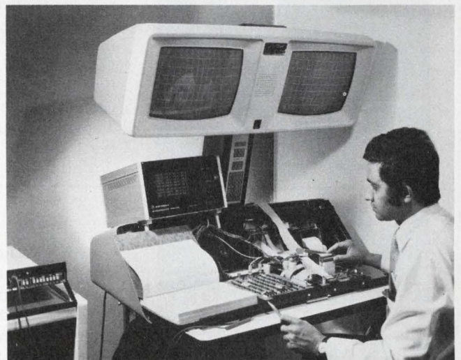
Motorola's MPA-1 analyzer works with the 8080 or 6800 and captures and displays 32 words in hex format. Status information can be ignored or captured and alternated with corresponding data.
