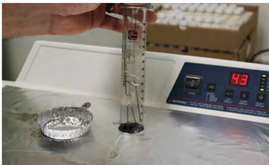
Figure 4. O-rings suspended in solvent, ready for insertion into a heated water bath.
