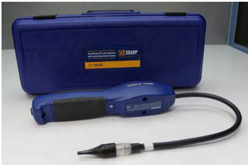
Figure 17. Hydrocarbon leak detector.
