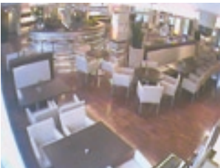
Perfect overview with a horizontal angle of view of 78° (3.6 mm focal length).
