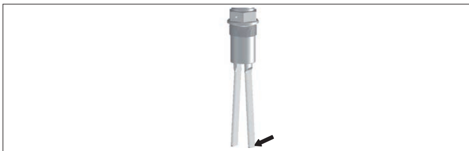
Fig. 26: Max. lateral load alongside fork side (narrow fork side)
