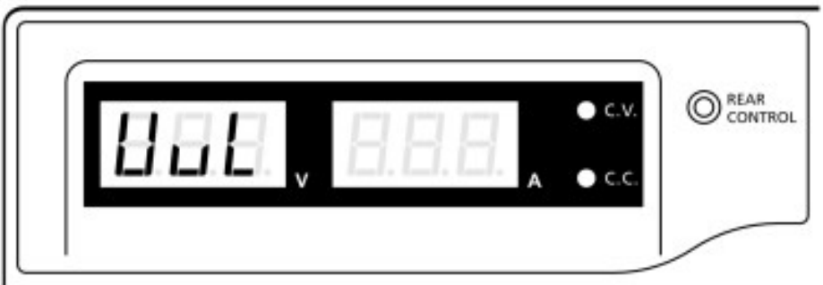
Figure 11 - Upper Voltage Limit
