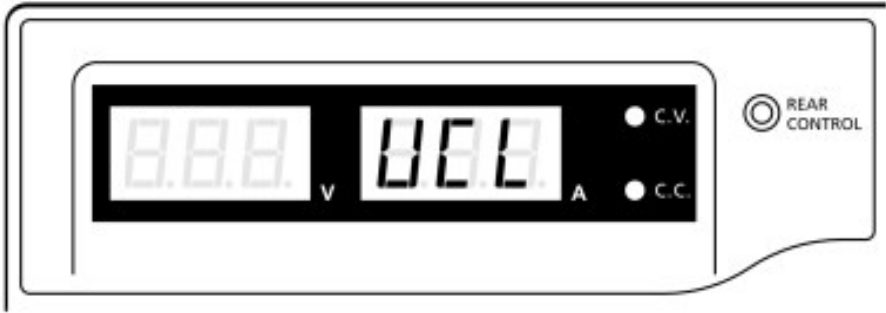
Figure 12 – Upper Current Limit
