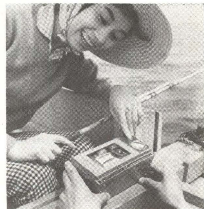
Nippon Electric calls this gadget a fish camera. It's a transistor sonar set. Frequency is 200 Kc, maximum depth 200 feet, price in Tokyo $110
