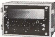
Far End Terminating Set Provides precision network termination during cable testing.
