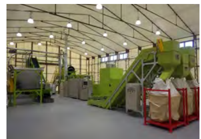
Near-infrared simultaneous sorting machine for three types of resin at CETEC
