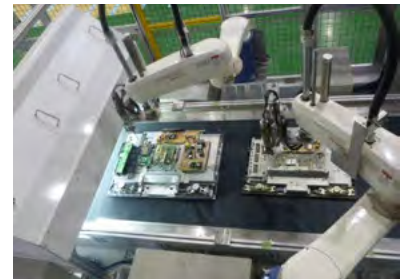
Automatic screw remover for flat screen TVs at PETECK
