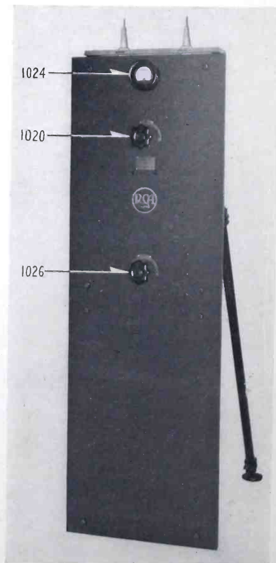
FIG. 16—ANTENNA TUNING AND COUPLING UNIT (Front View)
