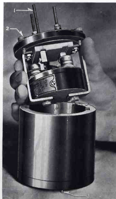
FIG. 2—PLACING CRYSTAL MOUNTING IN WELL
