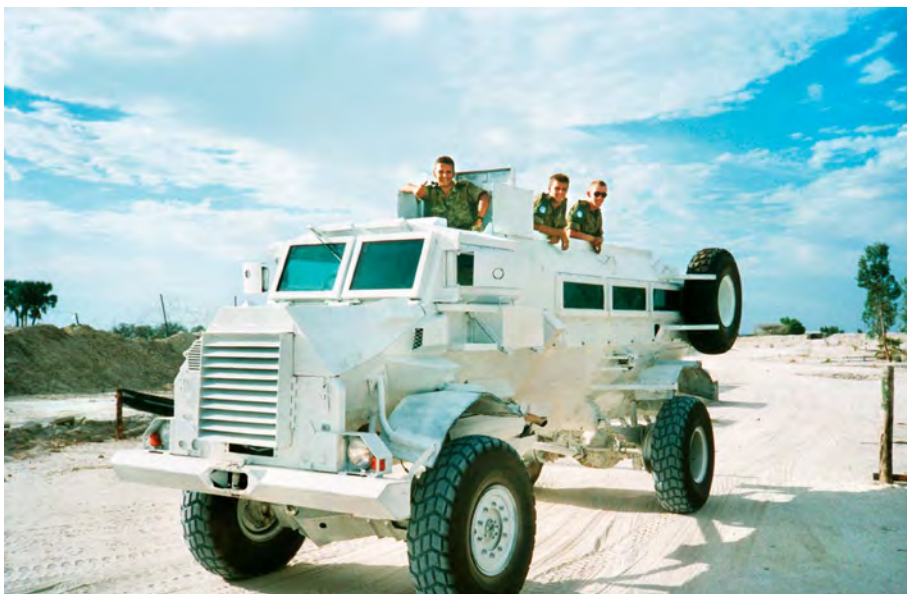
Australian members of the United Nations Transition Assistance Group aboard a South African-built Casspir armoured personnel carrier in Ondangwa, Namibia, in November 1989. Note the V-shaped hull. Photo: Australian War Memorial, Collection P01754.018, online .
