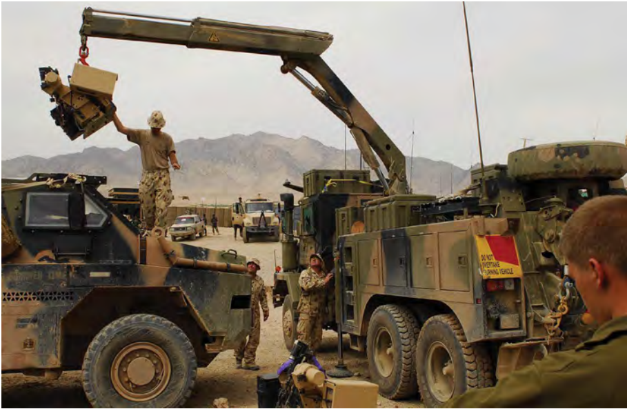
Australian Army engineers at a patrol base remove a remote weapons station from a Bushmaster for maintenance during operations near the village of Kakarak in southern Afghanistan in April 2009. Photo: Australian Department of Defence, online .
