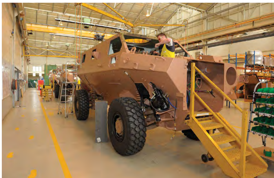
The V-shaped hull and monocoque construction are apparent on this Bushmaster under construction at the Thales plant in Bendigo, Victoria. Photo courtesy of Thales.
