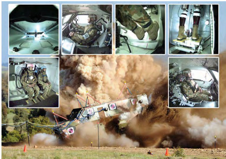
A Bushmaster that had seen action in Afghanistan, and its crew of military crash-test dummies, were selected for a violent experiment, designed by Defence scientists and Thales engineers, to examine the likely impact of a bomb on the vehicle and the soldiers aboard it. Photos: Australian Department of Defence.
