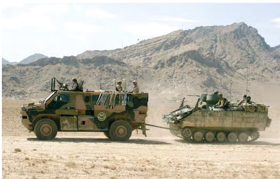
Wheels versus tracks? A Dutch Bushmaster towing a YPR near Tarin Kowt, Afghanistan, in August 2007. The YPR is an upgraded version of the American M113 armored personnel carrier used by the Dutch forces. Photo: Netherlands Ministry of Defence, online .
