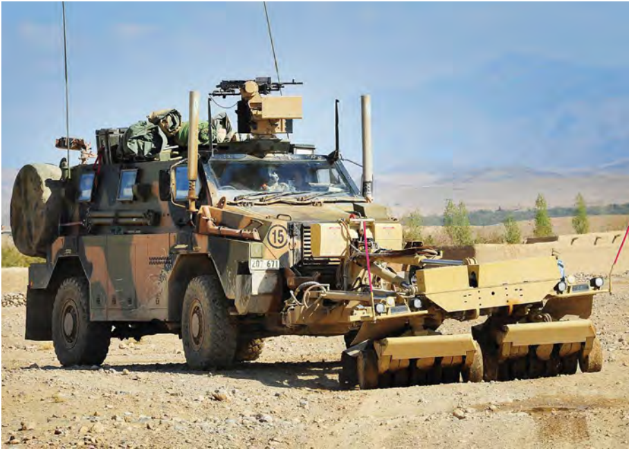
A Bushmaster with a self-protection adaptive roller kit (known as a 'SPARK roller') clearing roads of improvised explosive devices near Tarin Kowt, Afghanistan, in November 2012. Photo: Australian Department of Defence, online .
