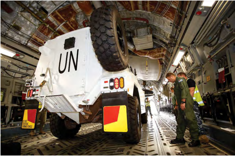
A Bushmaster is loaded onto a C-17 Globemaster at RAAF Base Amberley in southeast Queensland in March 2017 for delivery to Fijian peacekeepers on the Golan Heights. The giant transport aircraft can carry five Bushmasters, three Blackhawk helicopters, or up to 75 tonnes of equipment and supplies. Photo: Australian Department of Defence, online .
