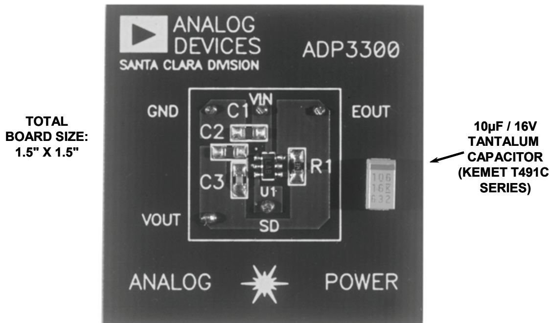
Figure 9.11: Size Does Make a Difference ADP3300 Evaluation Board
