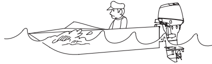
INCORRECT CAUSES BOAT TO "BOW STEER"
