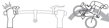
Figure 1.8: Apply both brakes together. Using the front brake only could cause the bike to pitch forward.
