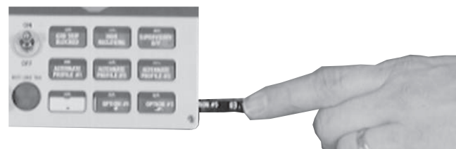
Figure 25. Labels are easily removed from and inserted into the operating panel
