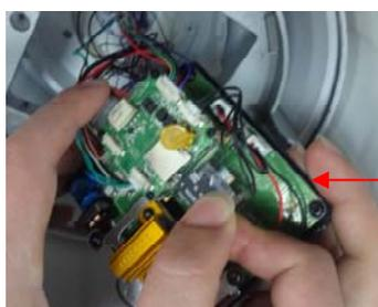
Insert Micro SD card following the direction shown in Figure 2-5
