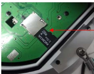
Insert Micro SD card following the direction shown in Figure 2-9
