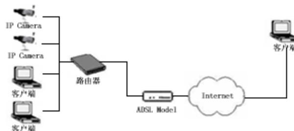
Users can set up DDNS domain name service at the same time. Fill the username and password which were applied in the DDNS server into the DDNS setting item, implement port mapping from the router. The router determines and points to the IP camera that need to be visited according to different ports, long-distance Internet user can visit the IP camera on the network via domain name directly.
