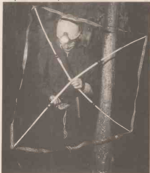
Surface signals being received underground using an inductive loop "aerial."
