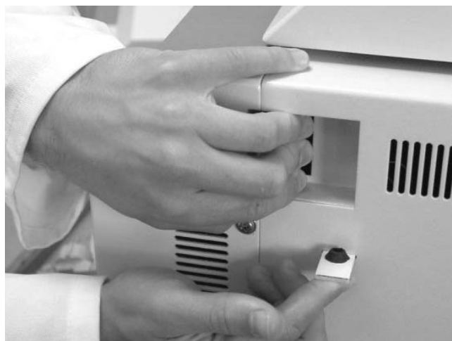
Figure 1. Insert the unlocking tool horizontally into the hole on the right hand side of the instrument.
