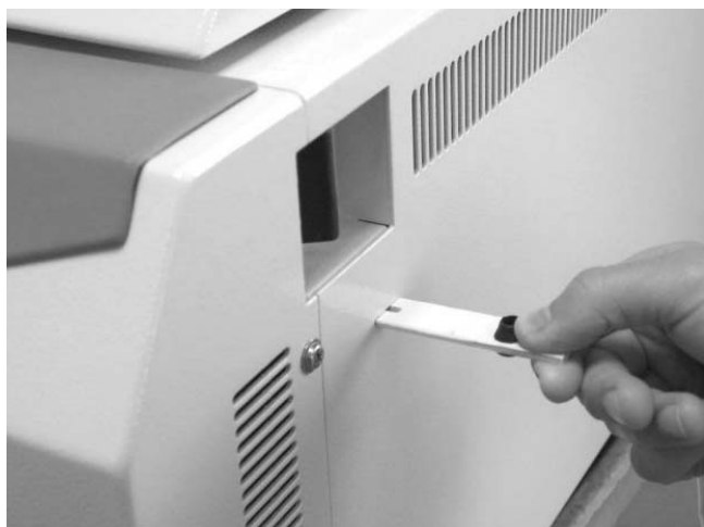
Figure 1. Insert the unlocking tool horizontally into the hole on the right hand side of the instrument.
