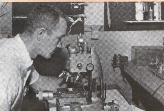
Toolmaker's microscope magnifies up to 1,000 times in turret lens, micrometer calibrated in .0001 inch.
