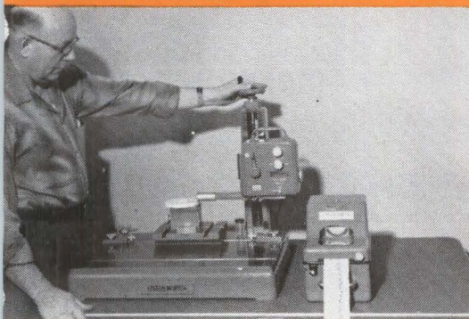
Talysurf electronically records the surface finish, amplified 50,000 times.
