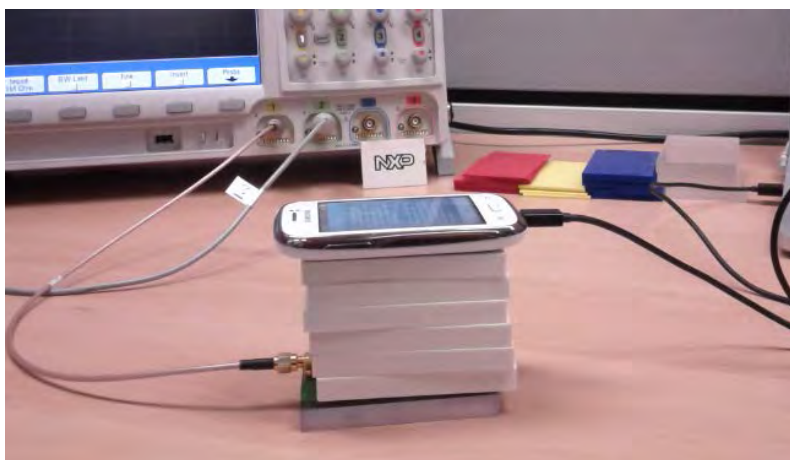
Fig 13. Recommended approach to spy RF activity
