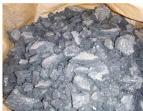
Sludge containing tungsten
