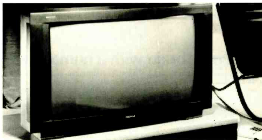
Fig. 3. Pal-plus pictures would be displayed on 16:9 widescreen TV sets similar to this current model for standard transmissions made by Nokia Consumer Electronics. (When standard 4:3 format pictures are shown on wide-screen sets the image can be expanded to fill the full width of the screen, though of course this cuts off some lines at the top and bottom).
