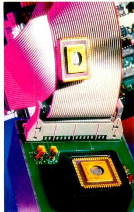
Programmable filter processor from SGS Thomson samples at 40MHz.
