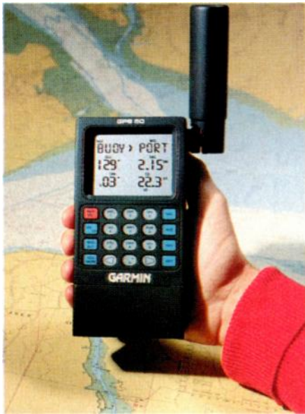
Know where you are to the nearest 100m. This handheld GPS set derives its position by phase triangulation from orbiting satellites. It costs about £1000
