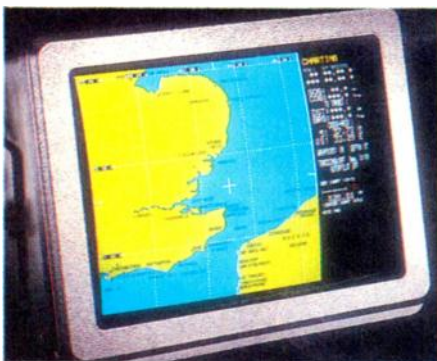
Digital processing and storage enables superimposition of chart information on the radar image
