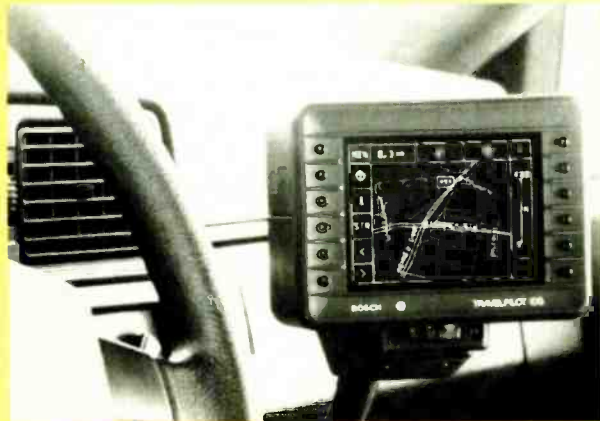
Vehicle navigation by dead reckoning: Bosch Travelpilot presents a route map stored in CD-rom and updates the car's position on the map by a mixture of magnetic bearing details, turn angles and distance travelled determined by data from the speedometer system.
