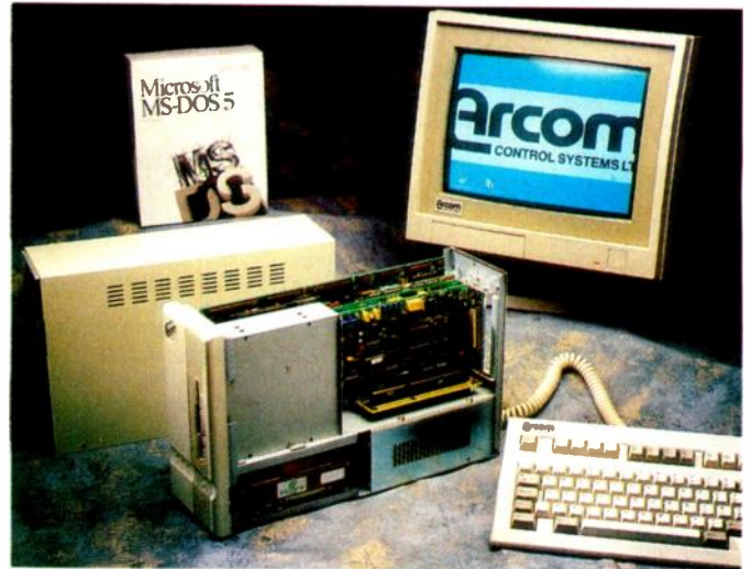
Arcom's 386 PC AT-compatible, which has a passive backplane and plug-CPU
