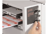
Fig. 7 Adjusting the retarder
