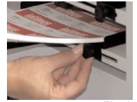
Fig. 6 Adjusting the paper guides
