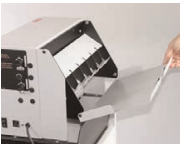
Fig. 4 Lowering the catch tray
