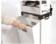
Fig. 16 Removing the waste box
