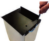
Fig. 2 Attaching cabinet top
