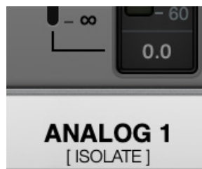
When active, the [ISOLATE] label is displayed below input channel labels
