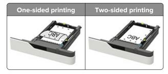
• Load envelopes with the flap side up and against the left side of the tray.
