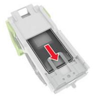
**Note:** If the staples are at the rear of the cartridge, then shake the cartridge downward to bring the staples near the metal bracket.
