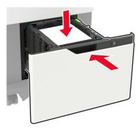
**6** From the control panel, set the paper size and paper type to match the paper loaded.
