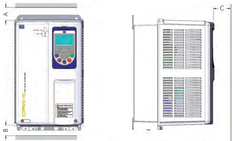
(a) Minimum top, bottom, and front clearance requirements for air circulation
