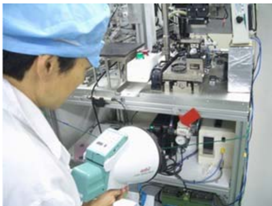
Measuring air leaks at points marked with arrows
