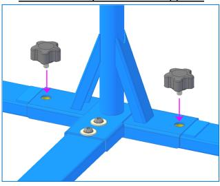
(4) Align tube holes and insert spring-knobs
