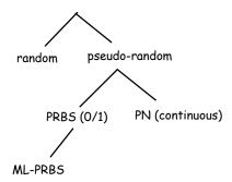
PN and PRBS signals have many important applications in communications systems. In this lecture we will study the properties of a type of PRBS called a maximal-length (ML) sequence, learn how to generate these sequences and look at one of their applications – "scrambling." Other applications include spread-spectrum systems and the generation of test signals.
