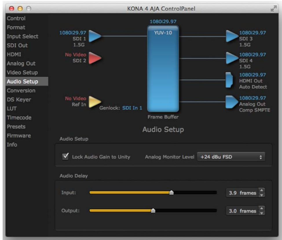
Figure 16. AJA Control Panel, Audio Setup Screen
