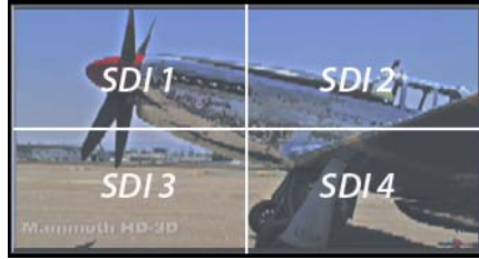
Figure 30. Mapping of Quad SDI Outputs
