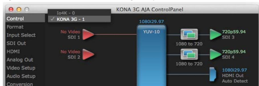
Figure 45. Control Panel Screen Showing Multiple AJA Devices
