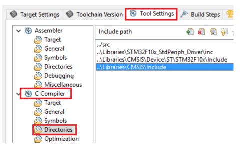
Figure 32 - C/C++ Include Path setting (start)
