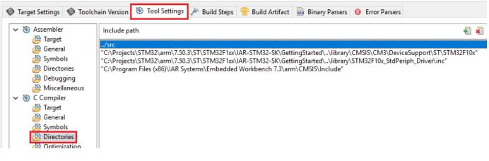
Figure 33 - C/C++ Include Path setting (end)
