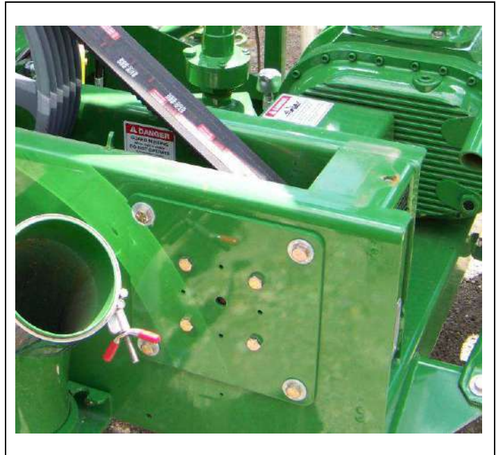
Fig. 5-20 Adjusting Anchor Bolts At Bearing Housing Assembly.
