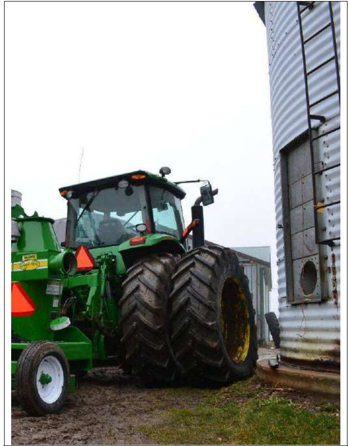
Fig. 4-8 Bin Clearance 8 ft
