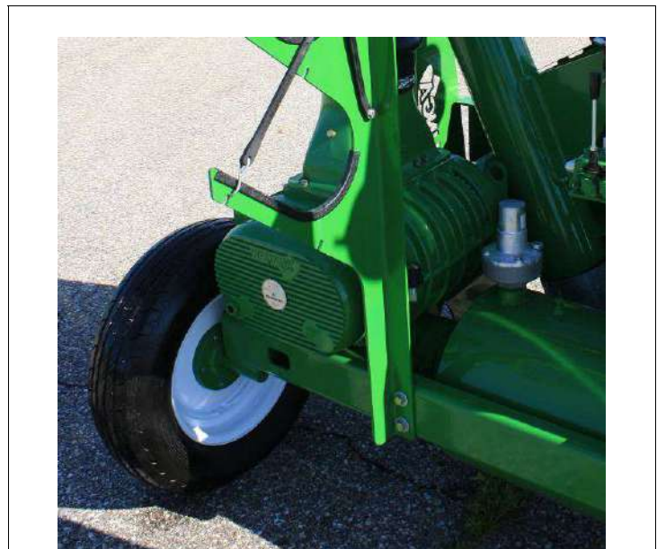
Fig. 5-5 Blower Reservoirs (Rear)
