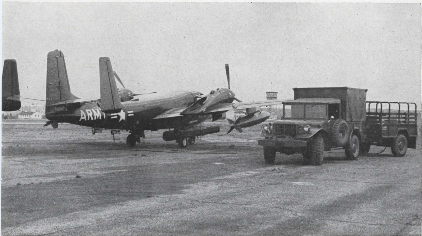
A truck containing the Mohawk adapter test unit (AN/ASM-88) drives up to an Army OV-1B to check its radar. No connection to the receiver or transmitter is necessary.
