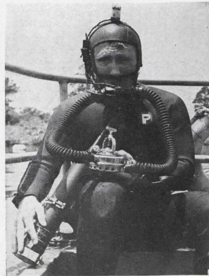
Aquasonics communicator is a 42-Kc a-m, device with 1,000 foot range
