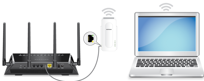
Figure 4. Extender in access point mode
