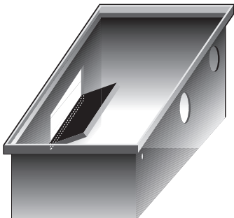
Fig. 21 Skimmer faceplate is properly placed when hinge is on the bottom.
