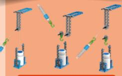
Pulleys Section Objective: Experiment to see how pulleys work like wheels and axles to reduce effort forces.
