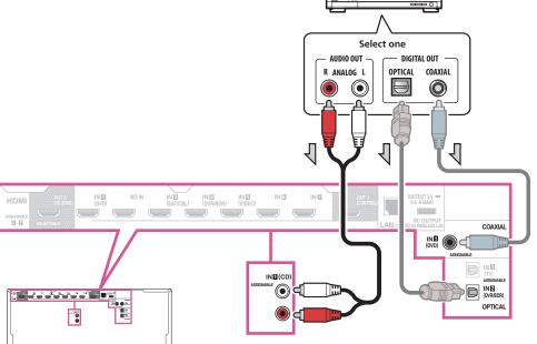
If your turntable has line-level outputs (i.e., it has a built-in phono pre-amp), connect it to the ANALOG IN 1
