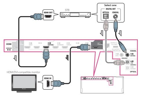
—If you use a digital audio cable or RCA (analog) audio cable, you'll need to tell the receiver which digital input you connected the set-top box to (see <a href="https://example.com/receiver-which digital">The Input Setup menu</a> on <a href="https://example.com/page 40">page 40</a>).
