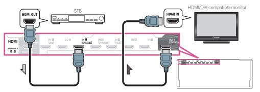
• Even if your set-top box is equipped with an HDMI output terminal, in some cases the sound is output from the digital audio output (optical or coaxial) and only the video is output from the HDMI output terminal. In this case, make the HDMI and digital audio connections as shown below.
