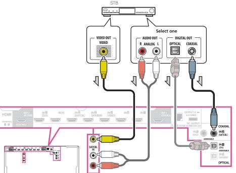
• If your set-top box is equipped with an HDMI output terminal, we recommend connecting it to the receiver's HDMI SAT/CBL IN terminal. When doing so, also connect the receiver and TV by HDMI (see Connecting using HDMI on page 26).
