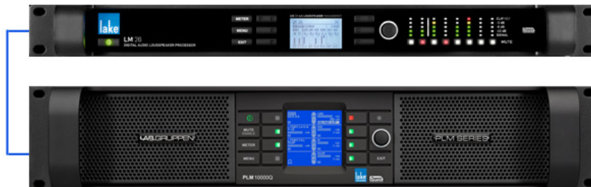
Figure 3-15: Only two Lake devices may be daisy chained for use with Dante
