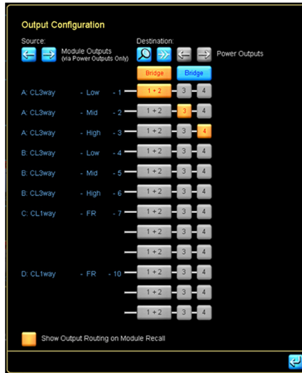
Figure 8-26: Bridge Mode (Lake-enabled amplifiers only)
