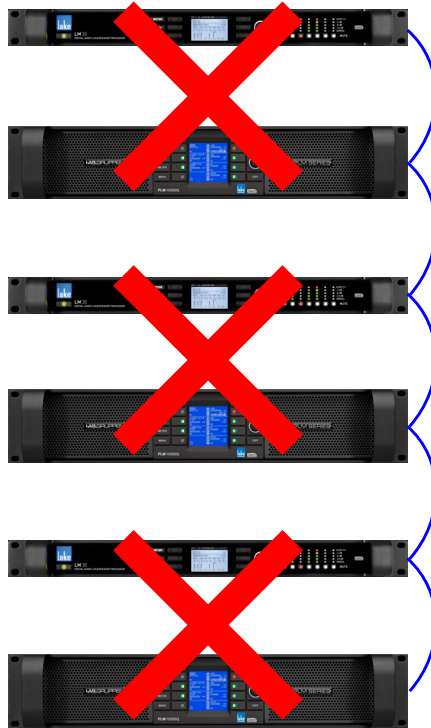
Figure 3-16: Do not daisy chain more than two Lake devices when using Dante
