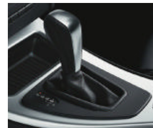
□ 6-speed STEPTRONIC automatic transmission provides a choice of three modes: "Drive" with Adaptive Transmission Control, "Sport" and STEPTRONIC automatic, for manual control without a clutch. Steering wheel-mounted paddle shifters are automatically added when ordered with Sport or M Sport Package.
