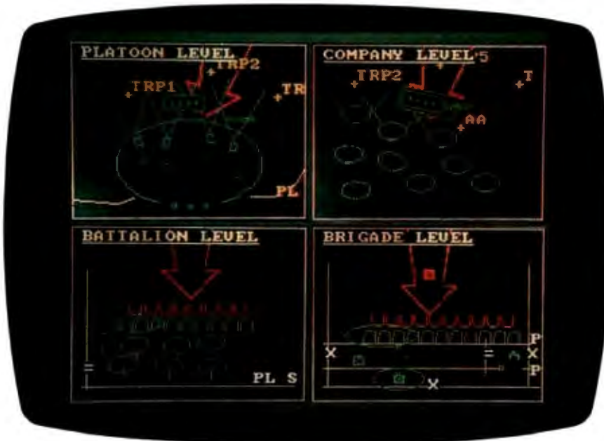
Photo 2: An example of a color display on a full-color EL prototype display from Planar Systems. (Photo courtesy of Planar Systems, Inc.)
