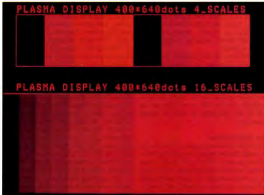
Photo 2: Gas-plasma displays can now display up to 16 levels of so-called "gray." (Photo courtesy of Panasonic Industrial Co.)
