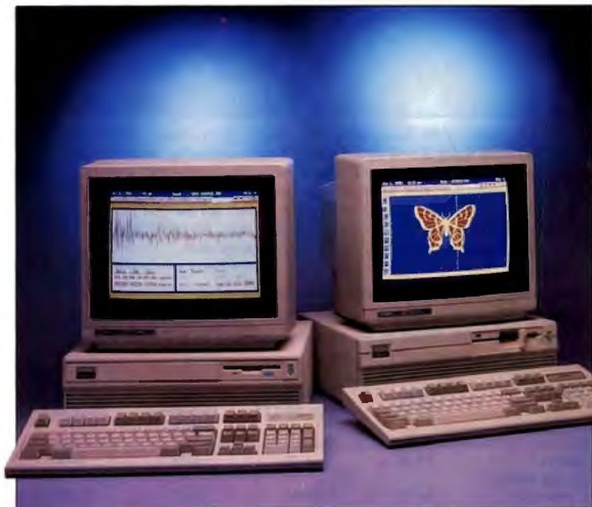
Two new low-end Tandy systems, the Tandy 1000 TL (left) and the 1000 SL (right). Both feature new sound capabilities. The TL is displaying a new application included with Tandy's DeskMate software, called Sound. The software lets you record, edit, and play back any captured audio sound. The SL is displaying a graphics application included with DeskMate.
