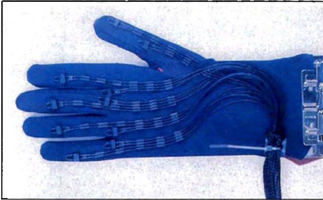
Photo 1: The DataGlove is a device that uses optical fiber sensors to measure and evaluate the range of joint movements, hyperextension, and abduction in the hand.
