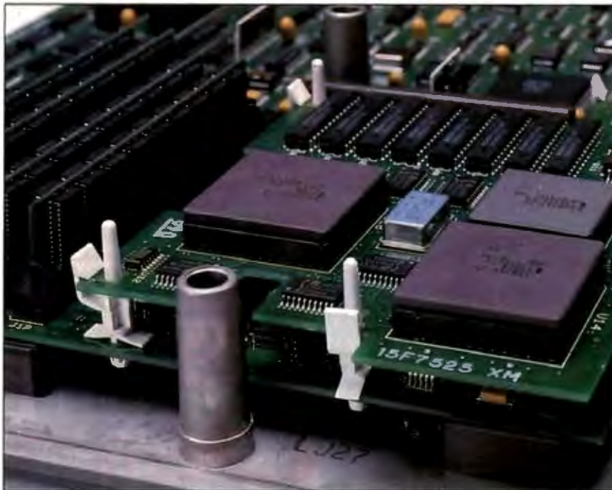
Photo 1: The inside of the IBM Model 70-A21. At the front, mounted on four white brackets, is the removable processor card. The 80386 CPU, 80387 NDP (if present), 82385 cache controller chip, and 64K bytes of cache RAM are located on this card. Immediately to the left of the processor card is 8 megabytes of SIMM-mounted system-board RAM.
