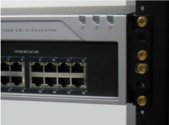
Figure 23: CX II/CXi II Controller Rack-Mount Installation - Fastening Angle Brackets to Rack Frame
