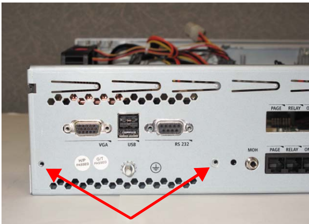
Figure 69: Retaining Hole Locations
