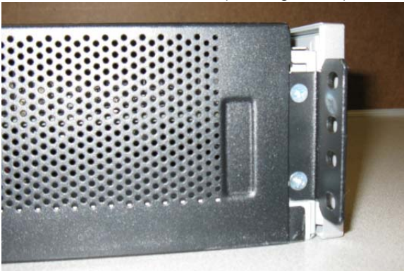
Figure 22: Figure 21: CX II/CXi II Controller Rack-Mount Installation - Attaching Brackets to Controller
