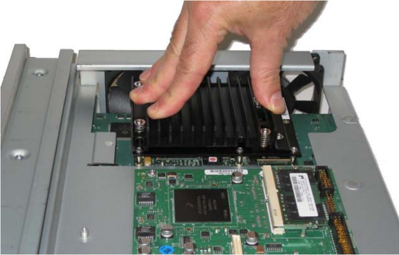
Figure 58: Installing an APC-MXe in the MXe Server
