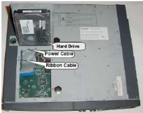
Figure 79: LX and 700-User Controller Hard Drive Installation
