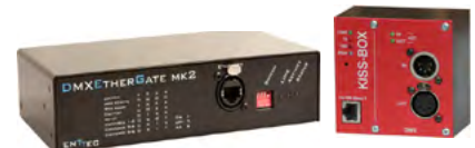
DMX-to-Ethernet adapters from Enttec and Kissbox.
