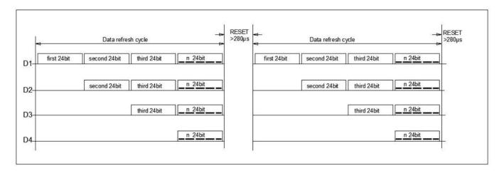
Note: The data of D1 is sent by MCU, D2, D3, D4 through pixel internal reshaping amplification to transmit.
