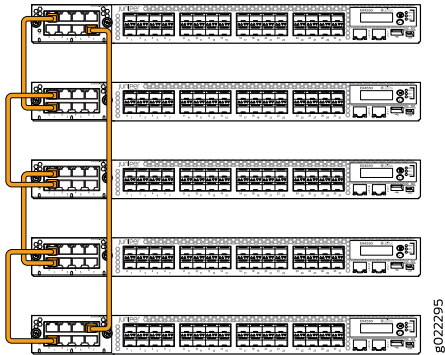
Figure 40: EX4550 Switches Mounted on a Single Rack and Connected in a Ring Topology Using 8-port 10GBASE-T Expansion Module and Using Short and Long Cables: Example 1
