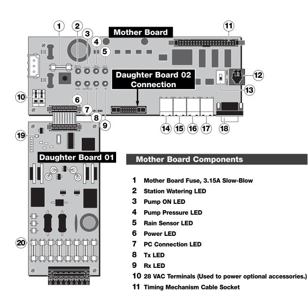
**14** (PC-Driven Models Only) Synchronization Terminal (Connect to second Gateway)
