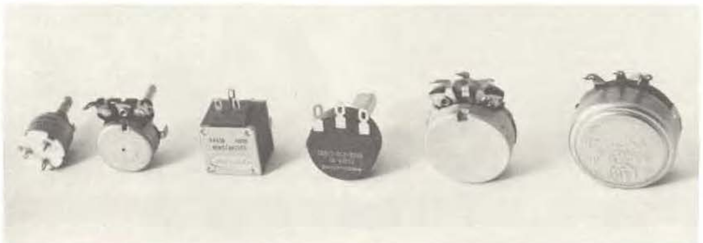
Fig. 8-5 Control potentiometer package selection guide
