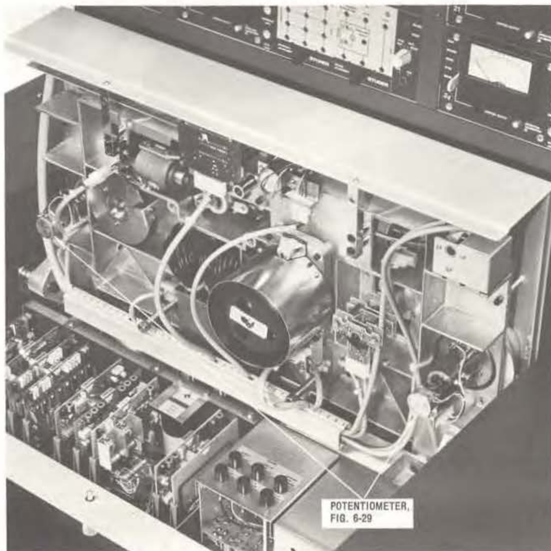
Fig. 6-30 View of underside of tape drive mechanics and electronics (Willi Studer, Switzerland)
