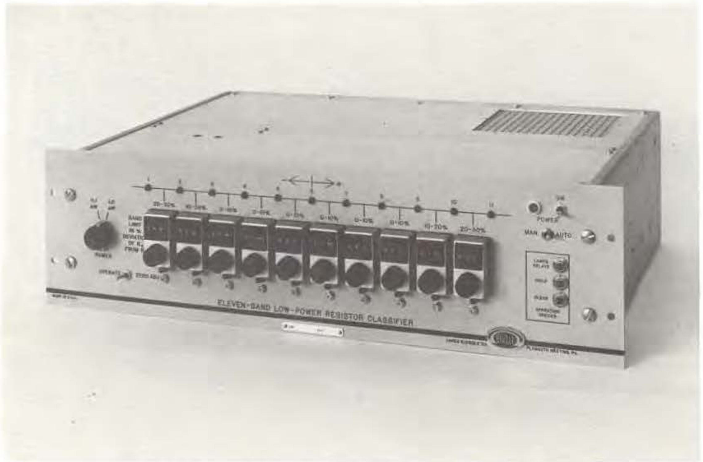
Fig. 6-27 A bridge used for high speed sorting of resistors and thermistors. (James G. Biddle Co.)
