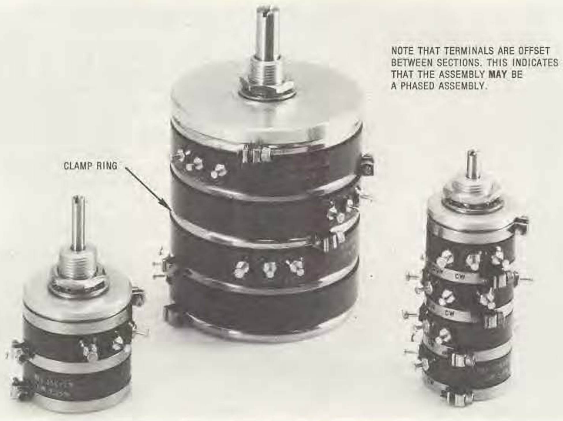
Fig. 6-16 Clamp ring style, phased potentiometer
