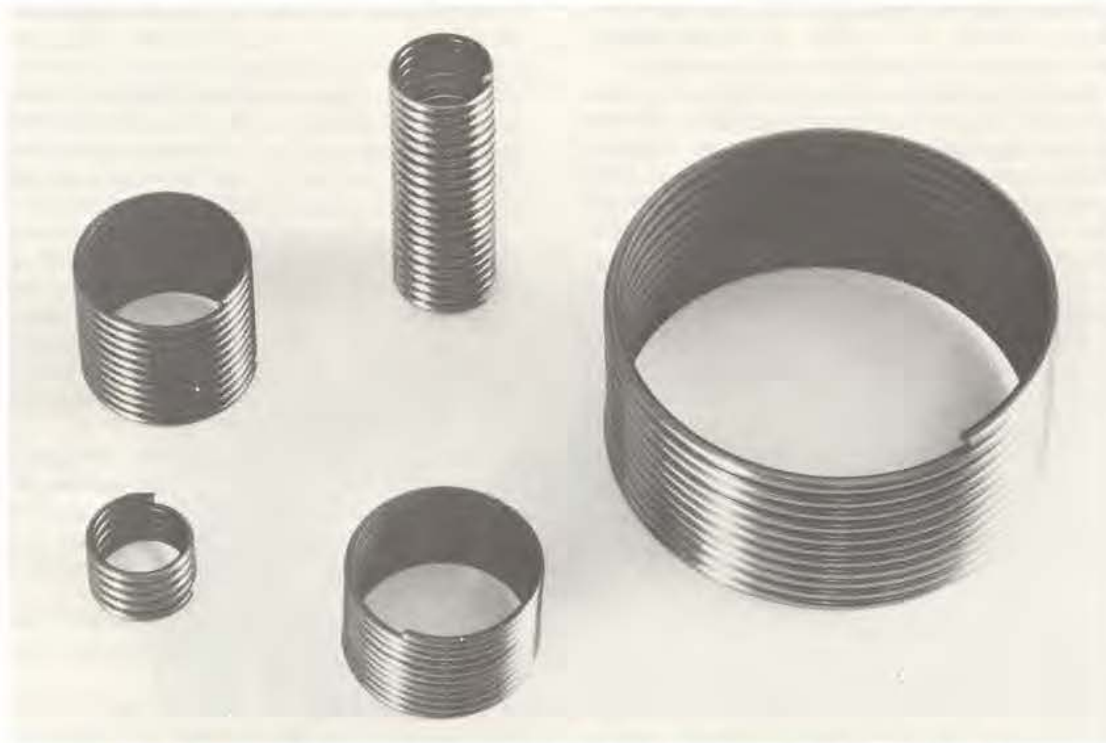
Fig. 7-11 A conductive plastic film is applied to an insulated mandrel to provide an element for a multi-turn potentiometer
