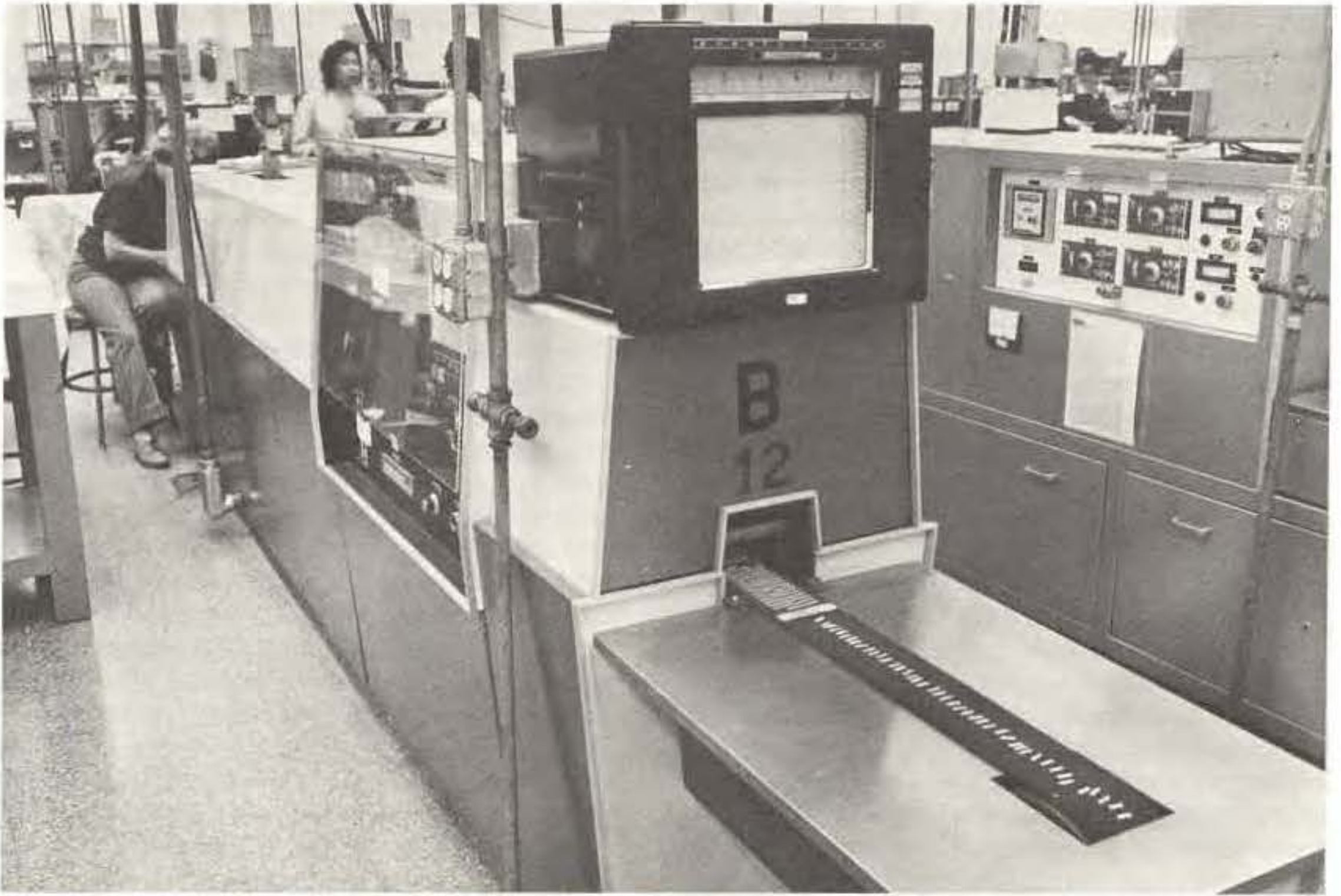
Fig. 7-9 The cermet ink is fired in a temperature controlled kiln
