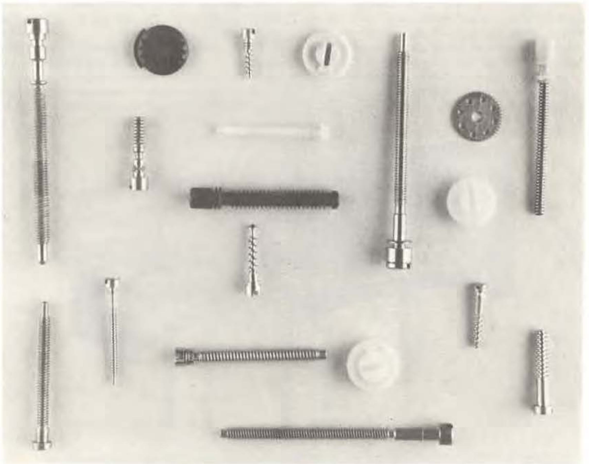
Fig. 7-29 Several typical rotary shaft actuators
