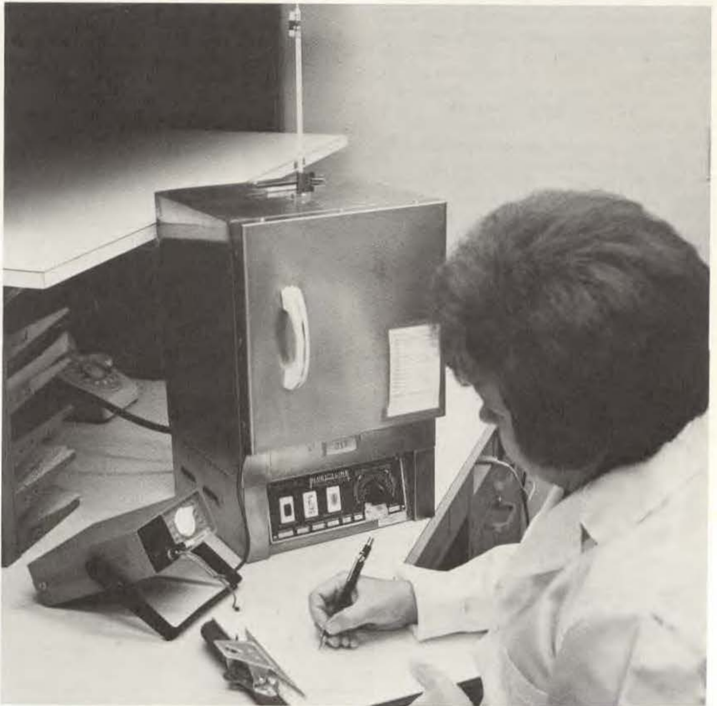
Fig. 2-25 Equipment configuration for temperature coefficient demonstration
