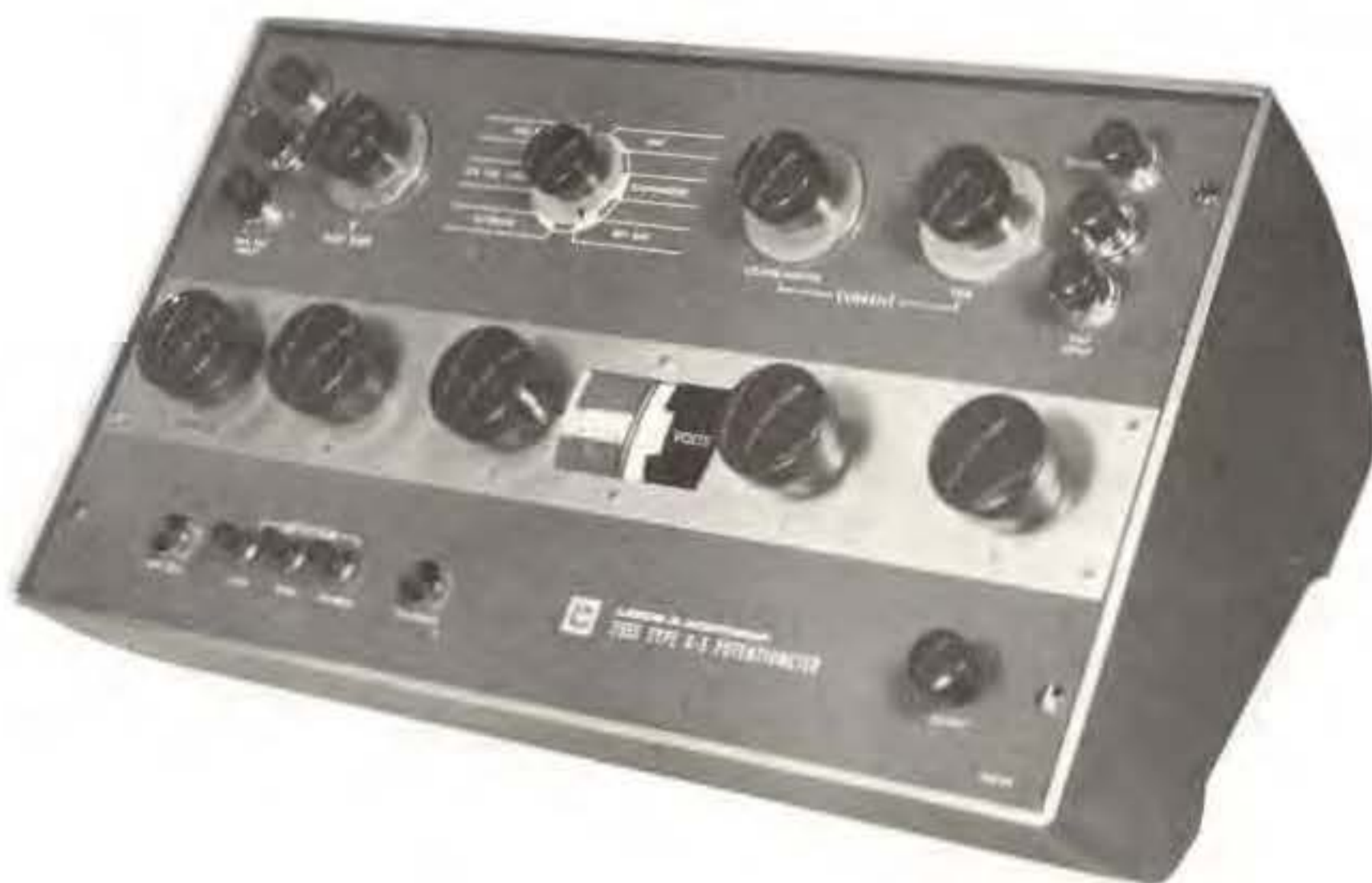
Fig. 1-6 Modern instrument for precision ratio measurement (Leeds & Northrup)
