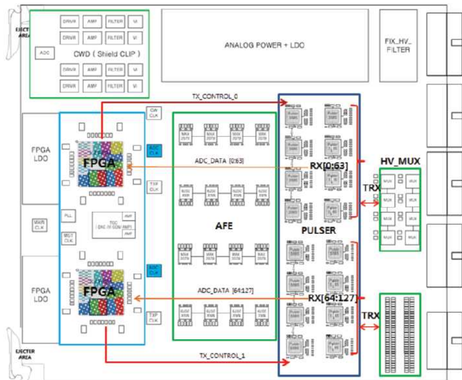
[Figure 5.8 BF Signal Flow]
