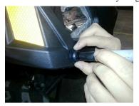
5. To mount the signal, first remove the rubber grommet from the light. Push the grommet into the hole until it is seeded correctly into the hole. Feed the wires of the light into the new hole you drilled. Notice the direction on the lens; make sure the "Top" is at the upper point of the light.
