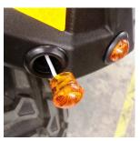
6. With the rear turn signals and tail/brake light in place, plug signals and tail/brake light into the wiring harness. (Both black wires from the signals connect to the orange (left) and blue (right) wires from harness. White wires from signals connect to the two long black wires coming from the rear of the harness.
